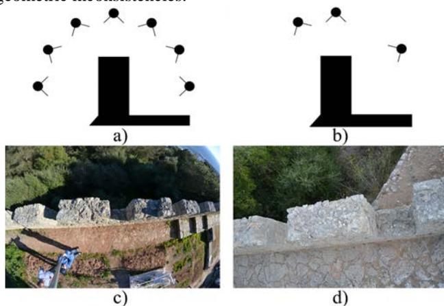
Fig. 1. a) Seven camera positions. b) Three camera positions. c) Fisheye image. d) Image taken with 18mm lens.
